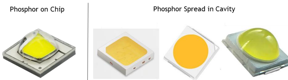
Figure 21 - Phosphor layer applied to the chip (left) vs. phosphor spread into the cavity of the LED as with typical flip chips.
