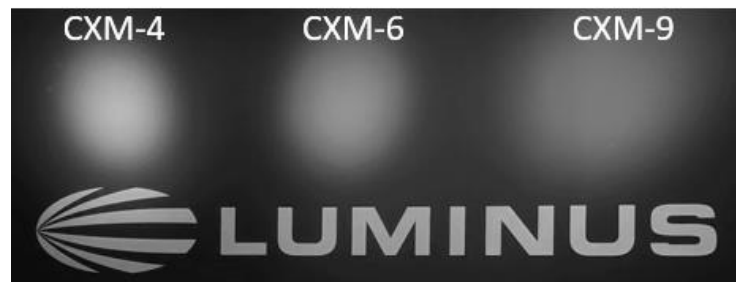
Figure 17 - Beam spots produced by Luminus Pico COB CXM-series LEDs. The smaller the source size (CXM-4, 4 mm), the smaller the beam angle and the higher the CBCP (brighter spot center).
